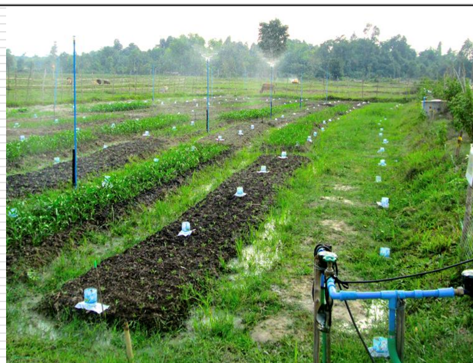
Figure 9: Experimental Units Installed with Spray Collectors
